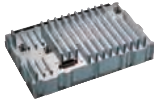
Power Amplifier Module of the Solid-State transceiver
